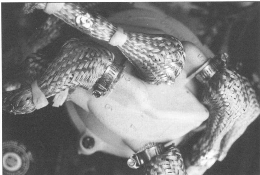
Fig 1—Braid installed over spark-plug wires at distributor.
