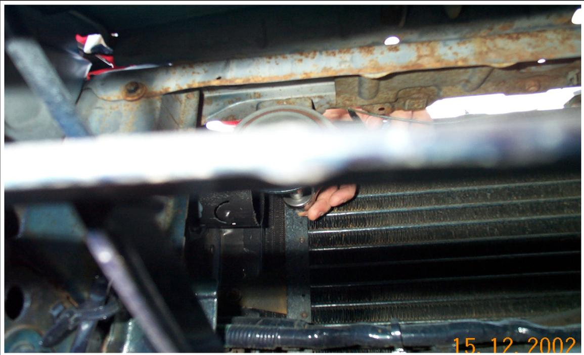
**Here you can see the horn on the passenger side - it's in our way so we must relocate it. We're going to lump it right next to the drivers' side horn.**
