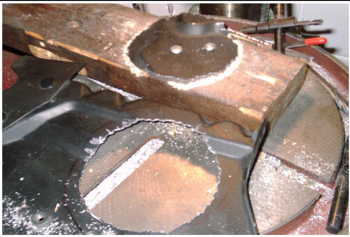
Here we used a metal routing bit to cut out the hole, but you can use a hacksaw blade if you want.
