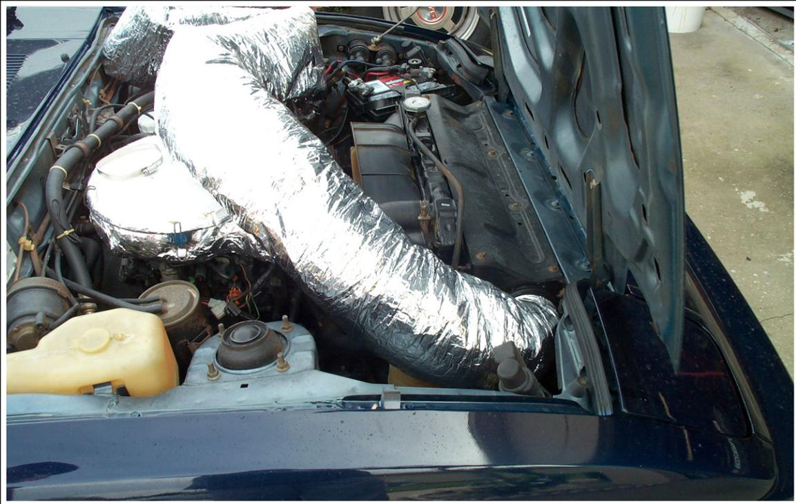
**Here we've attached the reinforced end to figure out how much additional ducting we'd need. Most stores don't sell the length you'd want, but around 2 feet seems to be the appropriate number. Better to have too much, than too little.**
