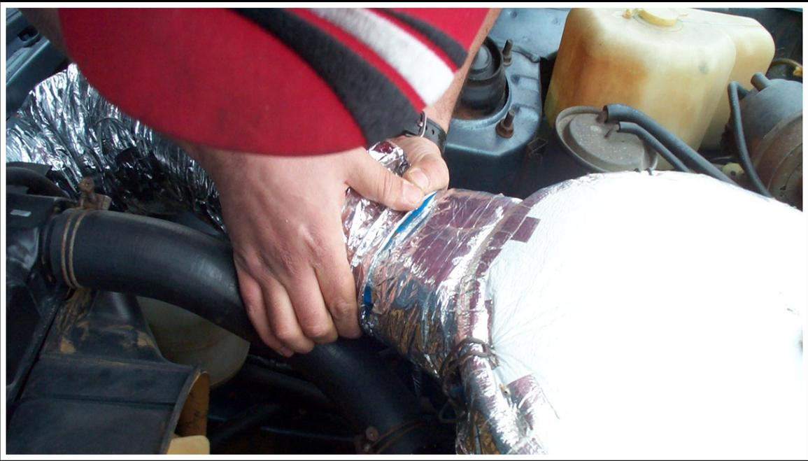
**Upon placing this end around the air cleaner housing, you'll find that it's not likely to hold on its own. Bring in the first 4 1/2" hose clamp!**
