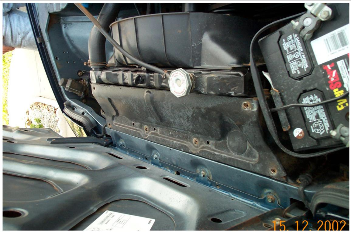
Remove the top radiator shroud. ( 6 10mm bolts)
