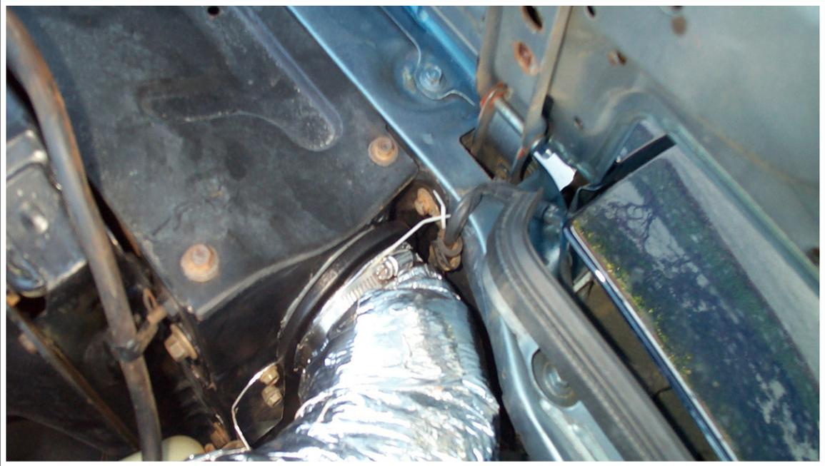
Secure this spot here with the 2nd 4 1/2" hose clamp, and now your Insulated Cold-Air Intake is complete. For additional heat soak protection, a heat shield over the intake manifold is a bonus. Enjoy your new, colder-fed engine!
